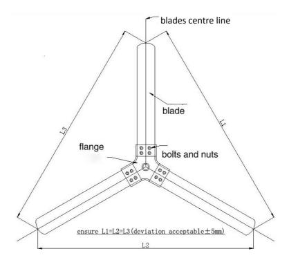
Note: if the distance between the tops of the blades in your installation exceeds the acceptable deviation, this may cause potential damages to the blades or flanges. If such damages are incurred, they will not be covered by the warranty.
