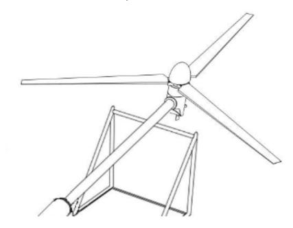
2. Fix the detachable part of the wind turbine connector to the top of tower by welding. Ensure that the centre line of the tower is parallel to the centre line of the casing when welding. Put the wind turbine head in the tower casing, and secure using the side screws.
