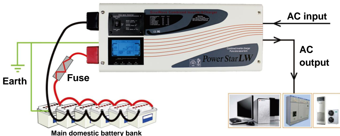
Wiring diagram for LK/LW Series Power Star inverters
